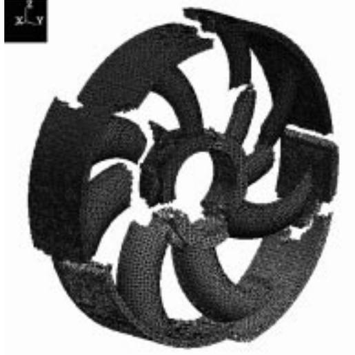
Figure 20: Finite element model of PROPELLER. Domain decomposition into six partitions.
