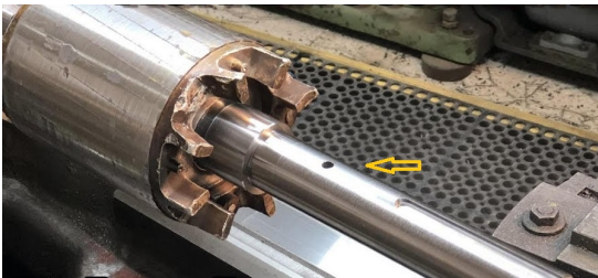
Fig. 7.21. Example of boundary conditions: shaft with a through-hole loaded by torque.
