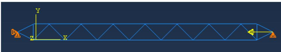
Fig. 14.5. Thompson-Hunt truss strut.
