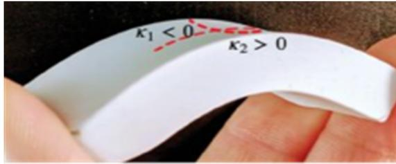
**Fig. 4.5.** Bent eraser. Note the anticlastic surface at the top. This is caused by the Poisson effect. The shape of the cross sectional area is no longer a simple rectangle.
