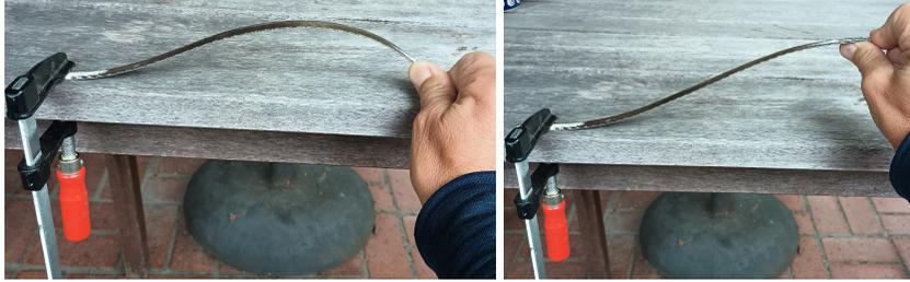
**Fig. 2.7.** Flexible piece of metal (metal saw blade) forced into two different shapes by applied forces and torques.
