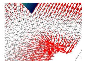
${\bf Fig.~9.2.}$  The effect of a reentrant corner on the flux: close-up.
