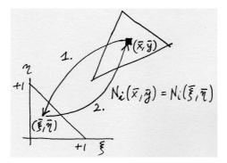
Fig. 5.7. Using the map from the standard triangle to evaluate basis functions over a general triangle
