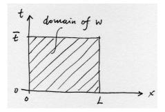
Fig. 1.3. The domain of the deflection function w
