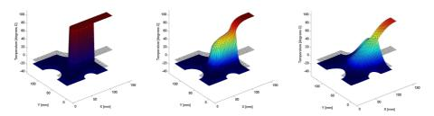
Fig. 9.5. Transient cooling of a shrink-fitted assembly; left to right: temperature distribution for time t=0,2,13
