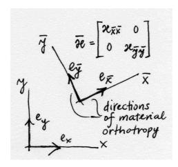
Fig. 5.10. Directions of material orthotropy
