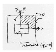
Fig. 6.1. Heat diffusion in a thick-walled rectangular tube
