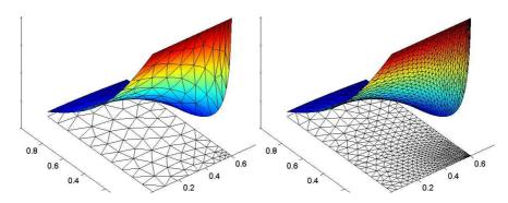
${\bf Fig.~9.3.}~{\rm T4~NAFEMS}$  Benchmark: solution with quadratic elements, initial and final mesh.
