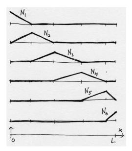
Fig. 2.5. Piecewise linear basis functions
