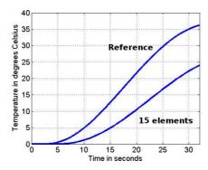
Fig. 7.2. Heat diffusion through a plate (one-dimensional problem): temperature  $0.02~\mathrm{m}$  under the heated face
