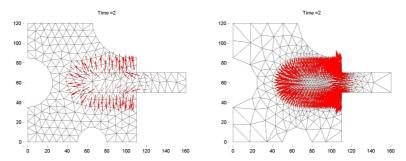
Fig. 9.6. Transient cooling of a shrink-fitted assembly; left: coarse mesh, right: adaptive mesh. Heat flux for time t=2
