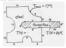
Fig. 7.3. Transient cooling of a shrink-fitted assembly: schematic
