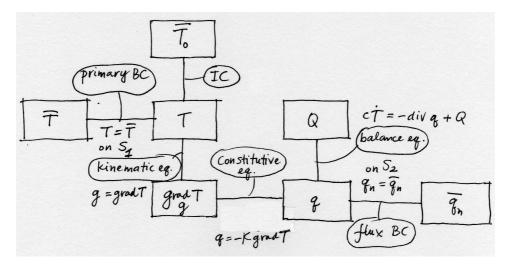
Fig. 4.3. Diagram of the heat conduction model
